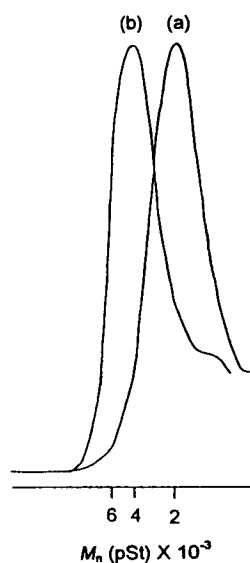
Fig. 2. GPC curves of (a) 2 and (b) 3 .
